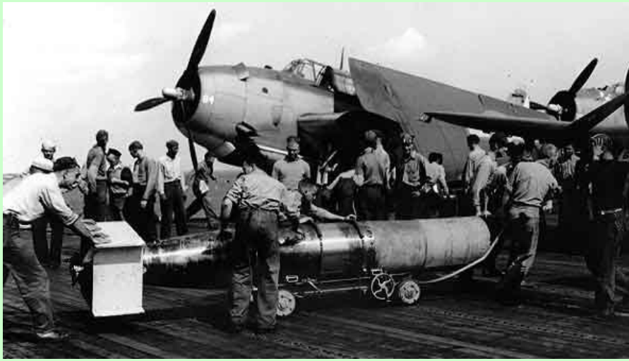
Modified Mk-13 torpedo being loaded in Wasp aircraft, circa 1944
